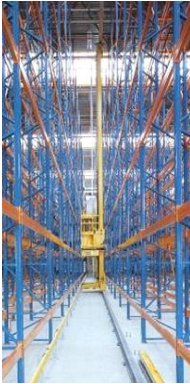
Figure 2C Crane operated racking: free standing and in “clad” rack
